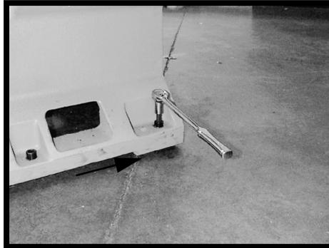
*Figure 3-19* Drive Down Corner Leveling Screws
