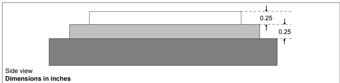
Dimension drawing of workpiece "The Raised Boss" (not to size).
