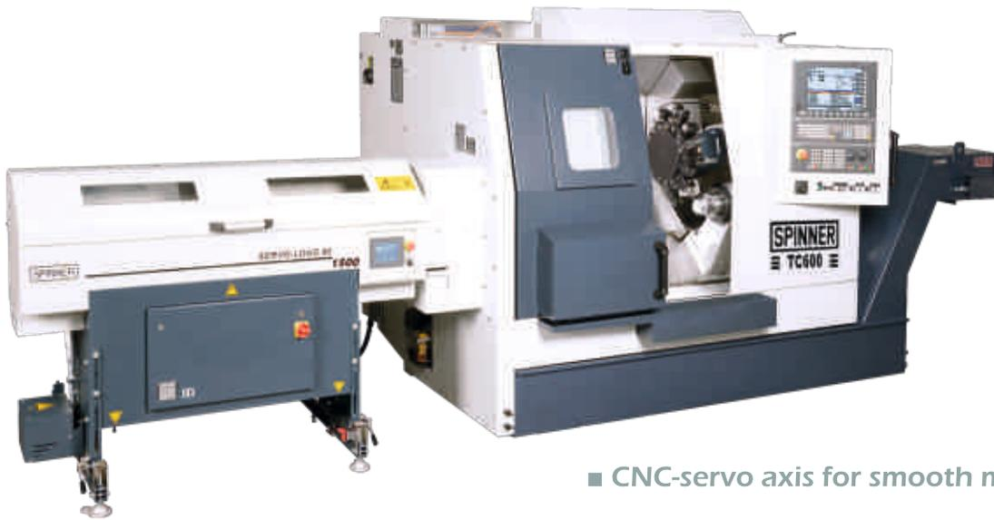
■ CNC-servo axis for smooth move of the bar
