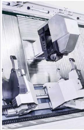
B-axis milling-turning head
