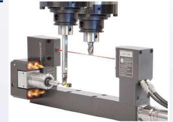
Combined tool setting system: non-contact measurement of rotating tools with laser ant touch probe for static tools
