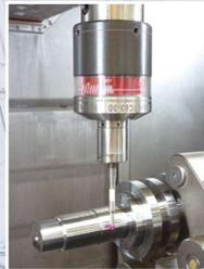
Touch probe for workpiece measuring
