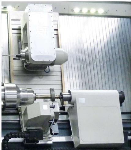
Turning-milling head with B axis
