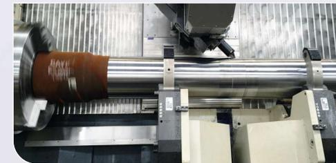
Pneumatic chuck with bore 360 mm (14.2")
