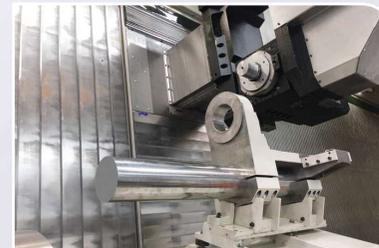
Boring bar holder mounted on the B-axis milling head. Parking position on the tailstock facilitates quick assembly.
