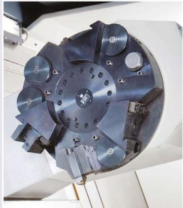
Special disc with slots for boring bars
