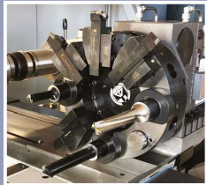
Disc turret for static tools
