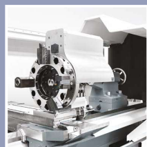
Turret for driven tools with C axis
