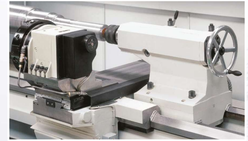
The standard tailstock has 125 mm (4.9") quill diameter. For heavy duty machining the diameter can be increased up to 140 mm (5.5") or 160 mm (6.3"). The quill is located in a specially extended body. Optionally the tailstock can be equipped with hydraulic quill, bearing system for the dead center, independent NC drive and hydraulic clamping system to the bed.
