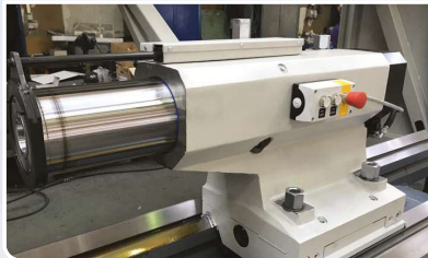
Tailstock with independent drive by push button
