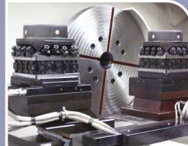
Combination of two 4-positions head-type turrets
