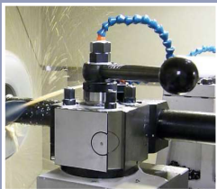
Parat toolpost with optional Capto seat
